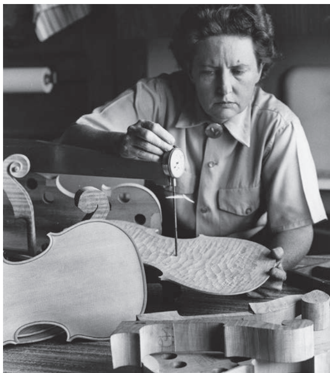
Measuring the thickness of a violin plate. Photo courtesy of the Hutchins estate.
