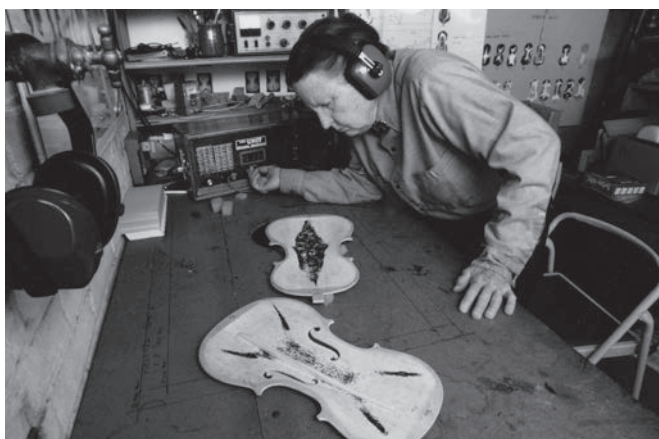
Hutchins using Chladni patterns to test a violin plate. Photo courtesy of the Hutchins estate.
